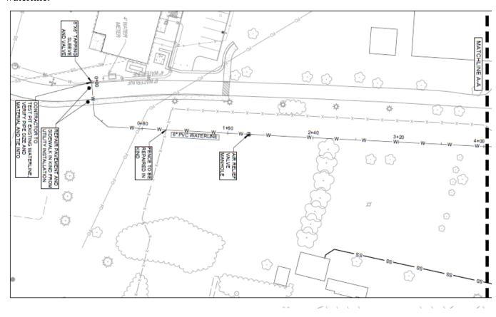
The second drawing shows the new waterline crossing the existing driveway and connecting at the south end of the new structure, near its loading dock area, with the new dining facility to the
